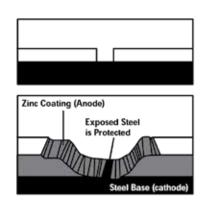
This is what happens to a scratch on galvanized steel. The zinc coating sacrifices itself slowly by galvanic action to protect the base steel. This sacrificial action continues as long as any zinc remains in the immediate area.
