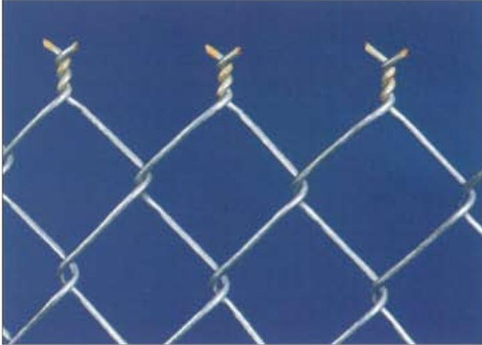
*Pre-coated fabric with uncoated tips. With pre-coated fabric, some manufacturers coat the bare ends, but many don't. No one coats the ends with the same material that protects the rest of the fabric.*
